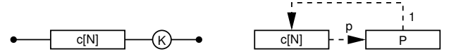
Figure 3: Generic OpenSESAME model for a k -of- N : G system with blocking failure propagation.
